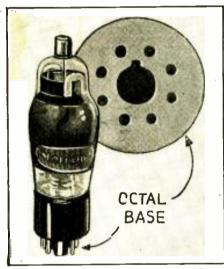
Fig. 8. The appearance of the new line of English octal-glass tubes.
